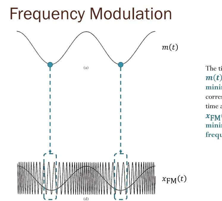
The time at which m(t) is at its minimum value corresponds to the time at which  $x_{FM}(t)$  has minimum frequency.
