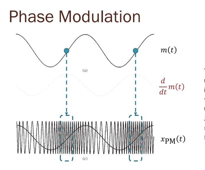
The time at which the **slope** of m(t)is at its **maximum** value corresponds to the time at which  $x_{PM}(t)$  has **maximum frequency**.
